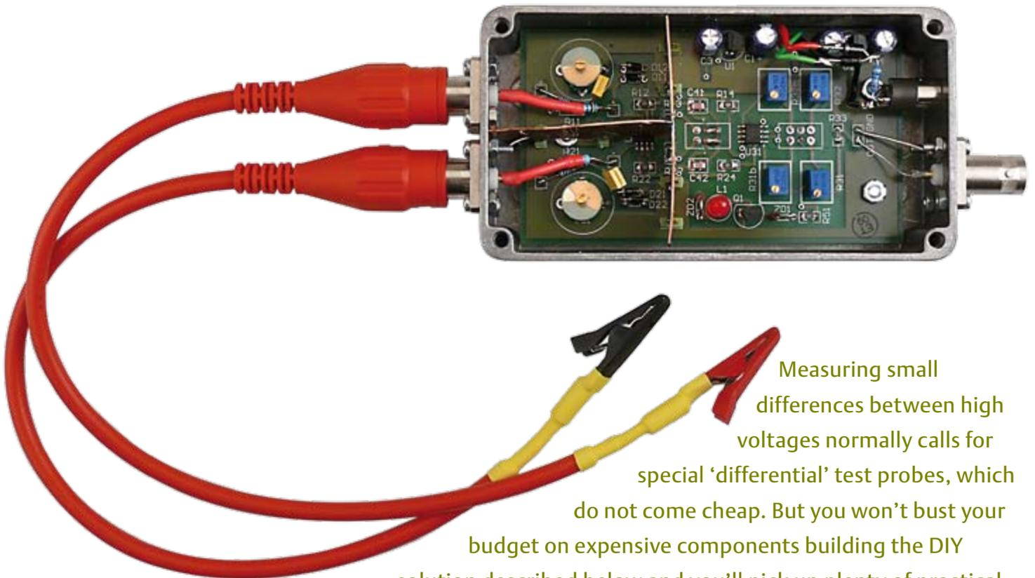
Measuring small differences between high voltages normally calls for special 'differential' test probes, which do not come cheap. But you won't bust your budget on expensive components building the DIY solution described below and you'll pick up plenty of practical know-how in the process.
