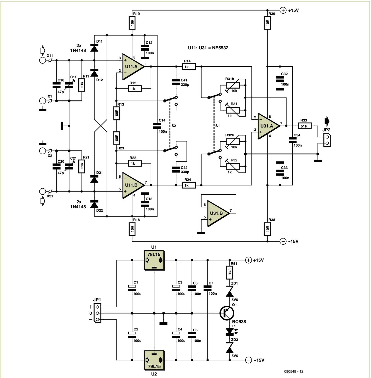
Figure 5. Full circuit (omitting the two 10 MΩ input resistors).
