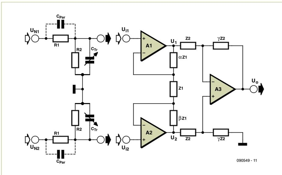
Figure 3. Block diagram with input attenuator (left) and instrumentation amplifier (right).
